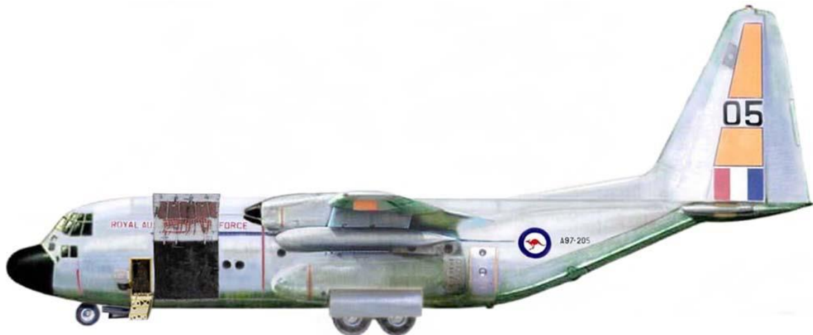
A97-205 with open crew and forward cargo doors – C-130A and C-130B had cargo doors, but discontinued for C-130E 21
