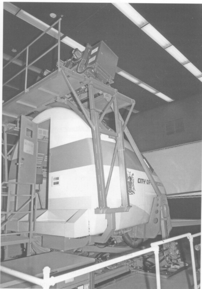
View of the exterior of Qantas Boeing 707 flight simulator No.2, showing the visual system display screen and the three image projectors mounted on top of the cockpit photo taken 1 April 1977
