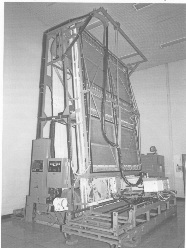
The belt-mounted terrain model and closed-circuit television camera of the visual system for the Boeing 707 flight simulator No.2 Image taken 23 February 1979
