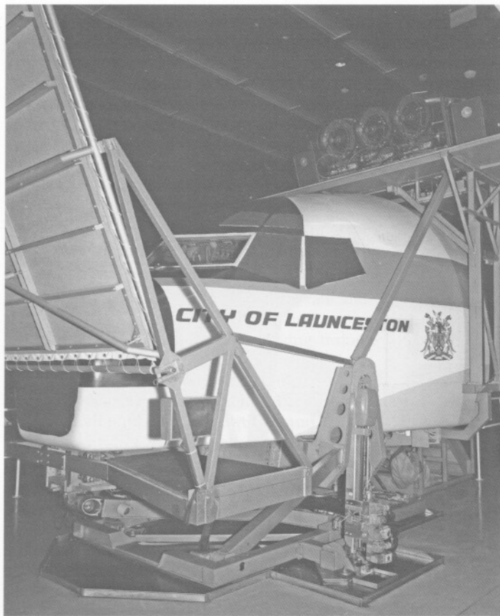
View of the exterior of Qantas Boeing 707 flight simulator No.2, showing the visual system display screen and the three image projectors mounted on top of the cockpit photo taken 1 April 1977
