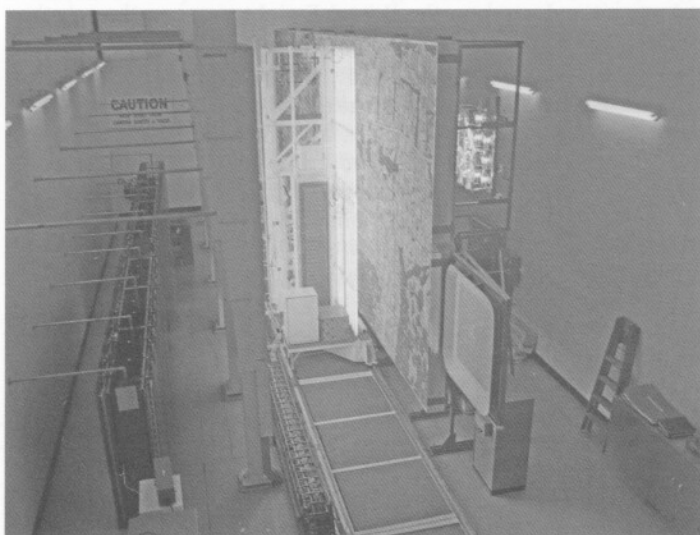
The 'daytime' map display which supported the No.2 Boeing 707 flight simulator and the No.1 Boeing 747 flight simulator. The video signals were switched between one machine and the other, although the crews in the B747 were reluctant to share with the B707 Image taken 11 December 1980
